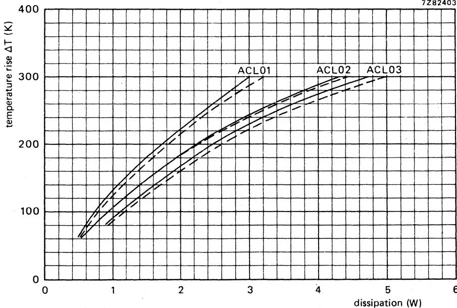
Fig. 3 Temperature rise of the resistor body as a function of the dissipation.
